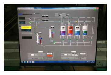
Cleaning of one lakh litre capacity silo is also done by computer. In ordinary systems, it is difficult to monitor cleaning and maintain quality standards. At dairy plant, all parameters such as concentration of cleaning agents and temperature of water to be used for
